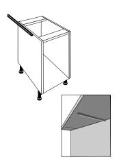
Support to the overhang can be achieved using L brackets, metal support bars screwed into the cabinets, or breakfast bar legs.  In the case of a handle-less kitchen, refer to the cabinet manufacturer's instructions regarding support and any additional battening requirements.
