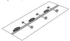
Use a jig with the correct size pocket profile for compact worktop connectors. Always refer to the jig manufacturer's guide before proceeding.
